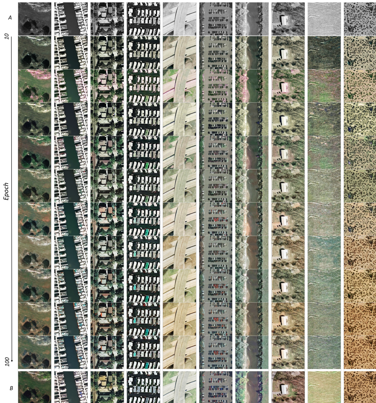
Figure 3: Examples of colorized aerial images using SpyncoGan along the training ( G_1(I) = O_{d_1}^{W \times H} ).
